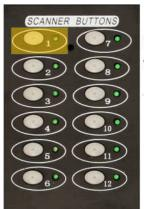
2. Select desired fixture, for example [1] LED PAR 9\*10 W with dmx address set to 001
